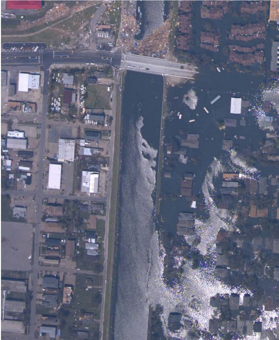
Fig. 1 Breach in the New Orleans 17th Street levee, August 31, 2006. The glint of the sun brightens the flood in places. U.S. National Oceanic and Atmospheric Administration photograph
